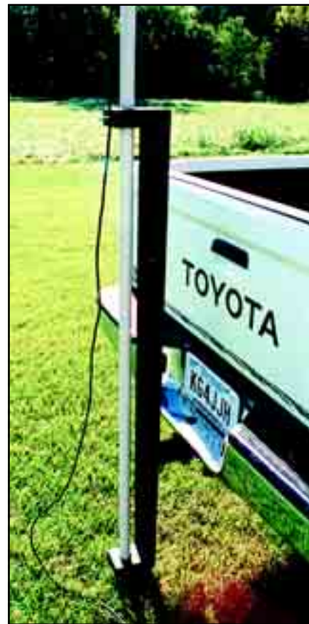
Figure 6—A view of the antenna mast support bracket.
