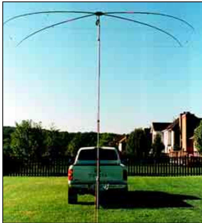
Figure 7—The erected antenna. In the air, the antenna resembles a black spider with its legs hanging down.
