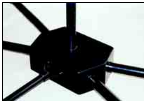
Figure 3—The center hub (left). Note the glued-in (epoxy) threaded sockets for the spreaders. The completed hub (right) shows the mounting stub extending upward and the feed line support extending to the lower left.
